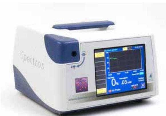
The T-Stat monitor with buccal probe and endoscopic catheter.
