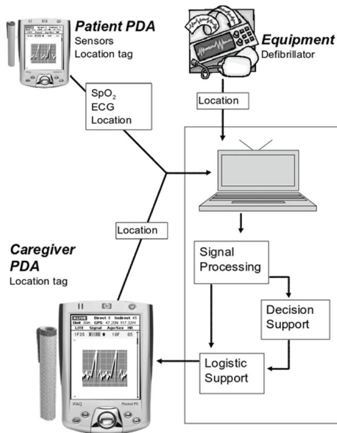
SMART components: Caregiver PDAs, location sensors and patients PDAs with ECG and SpO<sub>2</sub> sensors are wirelessly connected to SMART Central where all data are processed (1).
