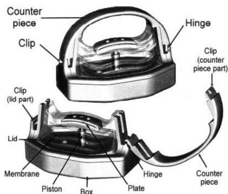
Left: FloWatch-PAB device in closed and open position (3)
