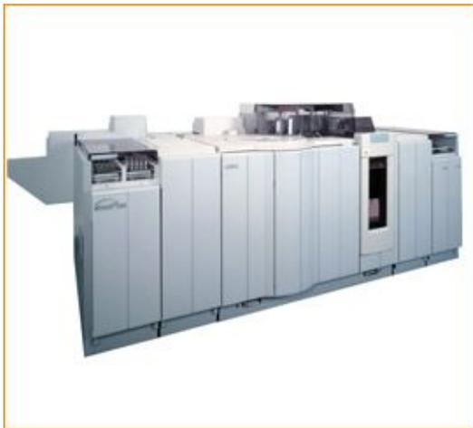
1010 model, a rapid-response, point-of-care system, is illustrated in Figure 1. This two-site assay uses two polyclonal antibodies, one labelled with biotin and the other with a ruthenium complex, that bind to NT-proBNP to form a sandwich (Lainchbury et al 2003). Streptavidin-coated microparticles are added to form a biotin-streptavidin complex, which enables detection and quantitation of NT-proBNP by chemiluminescence.
